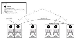
Figure 1. P-Grid overlay network
