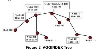
In an AGGINDEX tree, some sensors will have multiple identifiers, one being the so-called *real identifier*, or *r-id* which defines the data partition stored at this sensor. The
