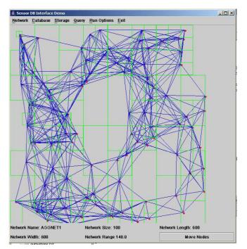
Figure 7. Network topology and partition by simulator. The solid lines represent network topology, and the rectangles show space partitioning.
